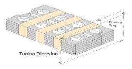
4.2) Tray stacking and taping: Each carton holds xx module trays and one empty tray.
